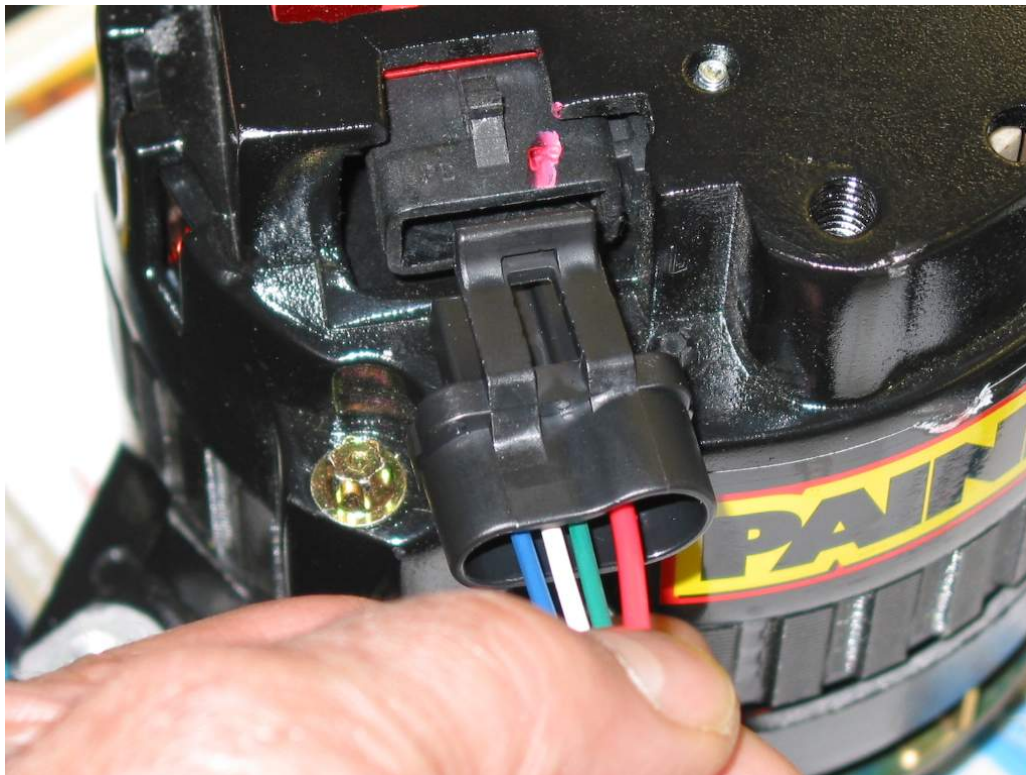
Photo 2 Installation Of Optional Plug Into Voltage Regulator
