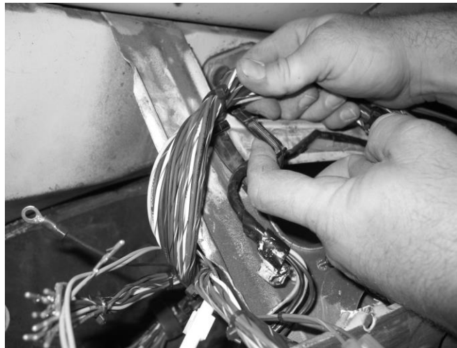
Figure 6-8 Steering Column Harness Clips
