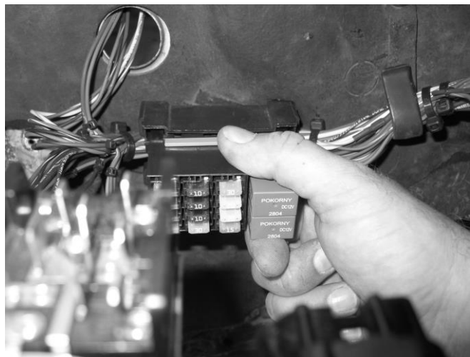
Figure 6-5 Snapping Fuse Block into Base
