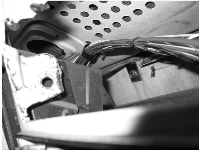
Figure 6-10 Original Harness Clips
