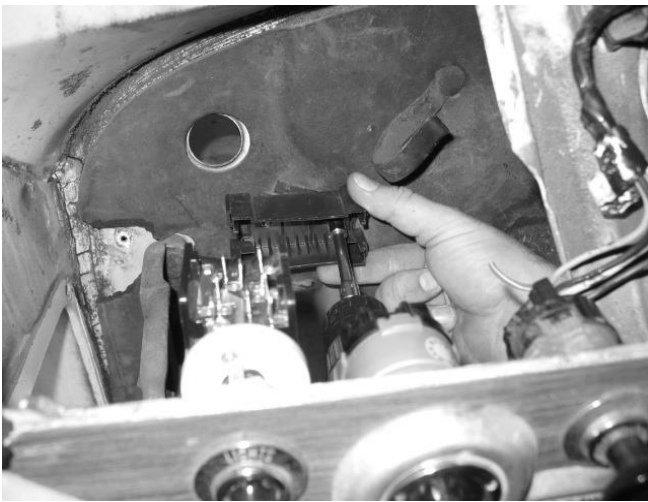
Figure 6-2 Fuse Block Base Position '67-'72
