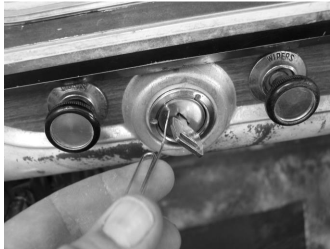
Step 2 – Bend open a paper clip and insert it into the small hole above the key. Notice the spring loaded pin.
