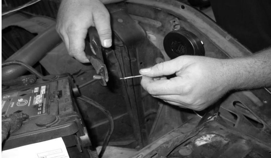
Figure 7-4 Horn Connections (All Models)
