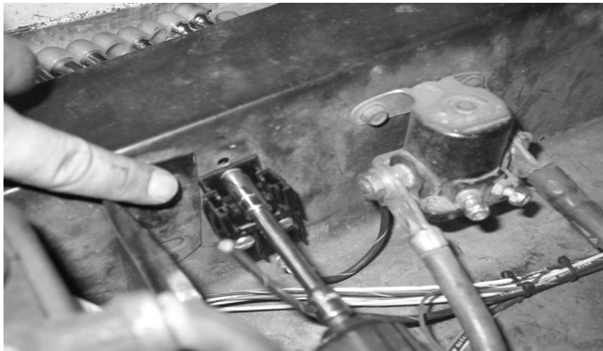
Figure 7-5 Installing the Maxi Fuse Holder '67-'72 Models
