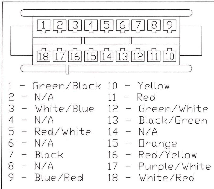
Figure 7-38 1973 - 1974 Cluster Pigtail Pinout
