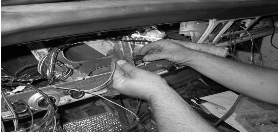
Figure 7-24 Cargo Light Connections
