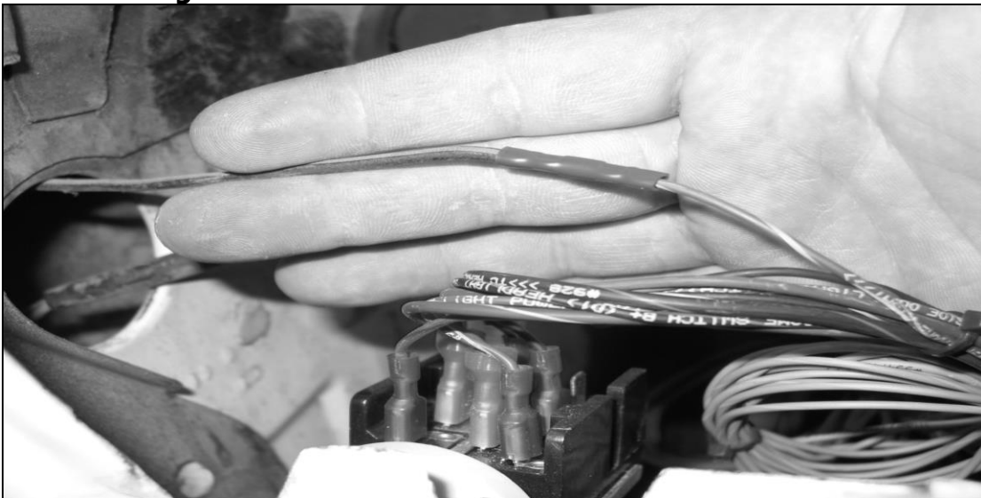
Figure 7-27 Dome Light Power Wire (All Models)
