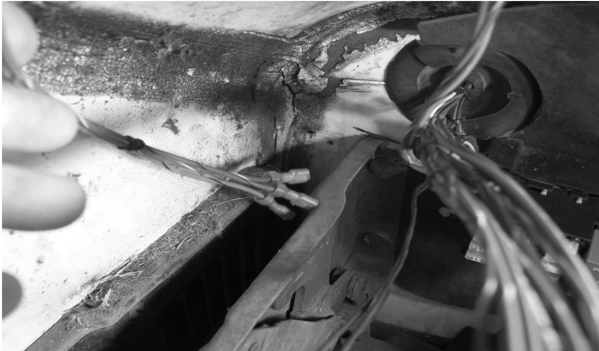
Figure 7-22 Routing the Dimmer Switch Wires
