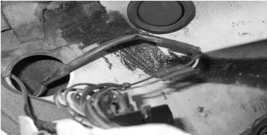
Figure 7-26 Door Jamb Switches – 1973-1977 Models
