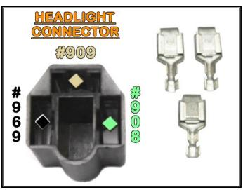
• The left/driver side headlamp connector(s) can now be plugged into the headlamp(s) and the headlamp(s) can now be installed into the grille.
