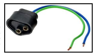
The factory, 2-wire regulator connector from the harness needs to be used. Due to a lack of usage by most customers, these connectors are not included with this Painless chassis harness. If you do not have these connectors, they can be obtained online, at a local auto parts store.
