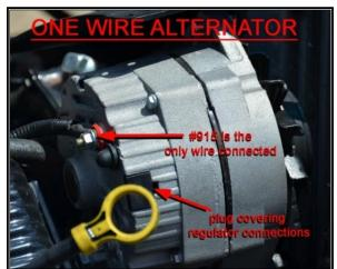
WHITE: 14-gauge wire, printed [START/CHARGE SECTION] #914 > ALTERNATOR REGULATOR EXCITER >, this is the indicator light wire and has switched ignition power from the fuse block. This wire will not be needed if you have a one-wire alternator.
