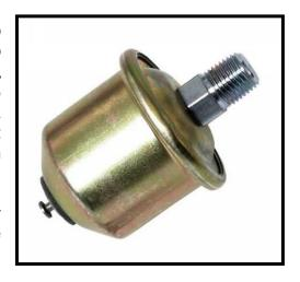
Route this LT. BLUE/BLACK #922 wire to the oil pressure sending unit, crimp-on the appropriate terminal for your connection, and connect.
