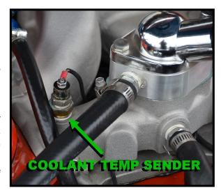
Route this LT. GREEN #921 wire to the coolant temp sensor, cut to length, strip ¼" insulation, and crimp on the appropriate terminal for your connection, and connect.
