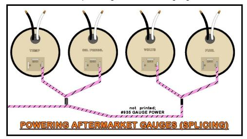
**#2)** Chaining or Jumpering- Run a PINK/BLACK #935 wire to a power post. Before terminating the wire with the proper terminal, insert another wire into the terminal and crimp. You now have 2 wires in 1 terminal. This additional wire then routes to the next gauge's power post. Before terminating that wire with the proper terminal, insert another wire into the terminal; and so on.
