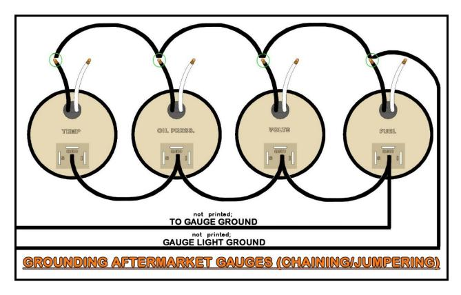
Gauge light power is supported by the **GRAY #930** wire. This wire connects to one of the leads for the gauge light or to the gauge light tab found on gauges with LED backlighting. To make these connections you can splice from this **GRAY #930** wire to all the gauges or chain/jumper it all together.
