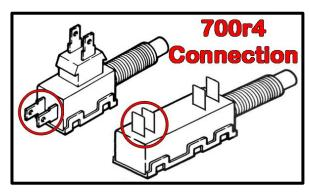
Two pins will be separate (or open) when the brakes are not applied. This is the pair of terminals further apart, closest to the plunger of the switch. When the brake is applied, these two pins will have contact with each other, or close. You will need these two posts that are normally open for brake light function.
