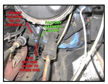
If you have dual fuel tanks, the **#939**, **#997**, & **#999** wires will need to be routed across the frame to the passenger side on the cross brace just behind the driver side door and not routed to the rear of the vehicle.
