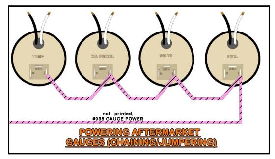
Grounds need to be supplied to the gauge lights and to any ground tab on the gauges. To make these ground connections you can splice from the provided ground wires to all the gauges or chain/jumper it all together. Both methods can be seen in the following two drawings:
