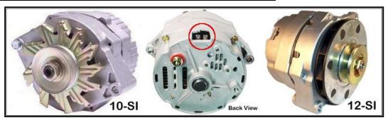
The 10-SI and 12-SI alternators are easy to identify. They have an external fan behind the pulley (the 12-SI has enclosed style fan blades) and a 2-pin connection. This 2-pin connection is circled on the second example in the image above. These are also commonly referred to as "Delco" or "Delcotron" alternators.
