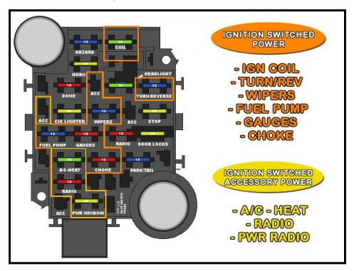
The drawing above shows all the switched ignition fuses. These fuses are powered by wires coming from the ignition switch (wires **#931**, **#932**, and **#933**) and receive power depending on what position the ignition switch is in. None of these fuses should have power when the ignition is in the *OFF* position. The <u>Ignition Switch Section</u> beginning on page 118 of this manual will go into further detail about power supplied to these fuses.
