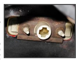
Using splices and heat shrink from the parts kit, connect the #926 and #927 wires to the lamp socket. Double up with the cut off piece of #926 with the #926 wire going to the socket. This allows connection to the front turn/park light as shown in the diagram below.
