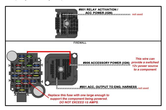
If a component is located in the engine compartment, connect #906 and #901 together. This will supply power to the #901 accessory wire in the <u>Headlight</u>
