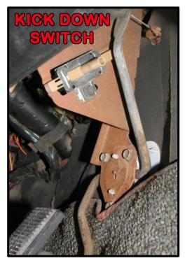
Connect a wire to each tab on the switch, it does not matter which wire goes where.
