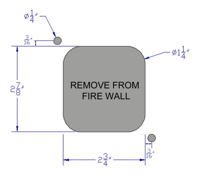
NOTE: This drawing MAY NOT be to scale, please double check your measurements with those on the drawing before any cutting or drilling.
