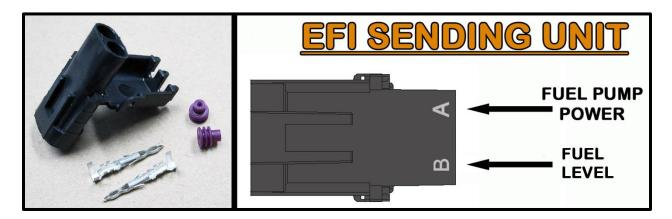
• The fuel pump wire in the above drawing will come from the output of a fuel pump relay, typically the "87" pin. DO NOT try to power a high pressure/high volume pump without a relay. Those using a Painless TBI harness, #60101/#60201 this will be a TAN/WHITE wire supplied by that harness. Those using one of our LS harnesses such as #60508 or one of our Gen III Vortec harnesses like #60217, this will be a gray wire supplied by those harnesses.
