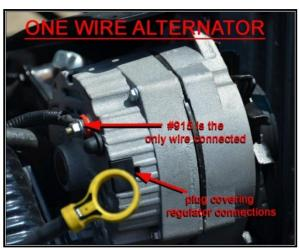
**POWER (BATTERY)**, this is the sense wire, it provides a battery power source, or voltage sense, that all voltage regulators require. This wire has power at all times and comes from the large battery supply splice in the harness. This wire will not be needed if you have a one wire alternator or a GM CS series alternator. See the various alternator illustrations on pages 60, 61, & 63 and the <a href="#">Charge/Battery Power Schematic</a> on page 68.
