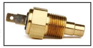
The coolant temp sending unit/switch can be mounted in the intake manifold or in the side of either cylinder head. These will have a peg, tab, or threaded post to connect to, as seen in the photos on this page. Terminals and a factory style connector have been supplied to allow connecting to a factory style sensor, rollover crimpers will be needed to properly install this terminal.
