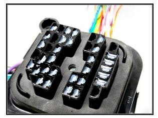
Using a <sup>3</sup>/<sub>8</sub>" socket, tighten the mounting thru bolt on the engine bulkhead to the firewall connector. DO NOT FORCE OR OVERTIGHTEN!
