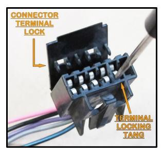
Using the picture below, insert the wiper switch wires of the Painless harness into your connector. The terminals will only fit into the connector one way.
