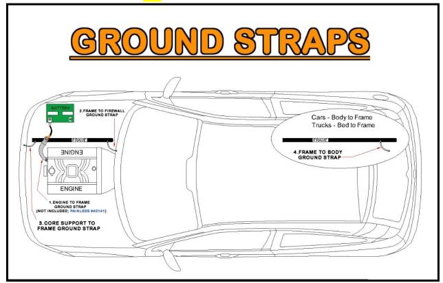
A ground is simply the common path electrical current follows back to the battery. A ground, or chassis ground as it is often called, is any bare metal surface found on the vehicle which is in turn connected back to the frame/negative side of the battery through mounting points and ground straps. Grounds are needed in order for the electrical current to complete the circuit.
