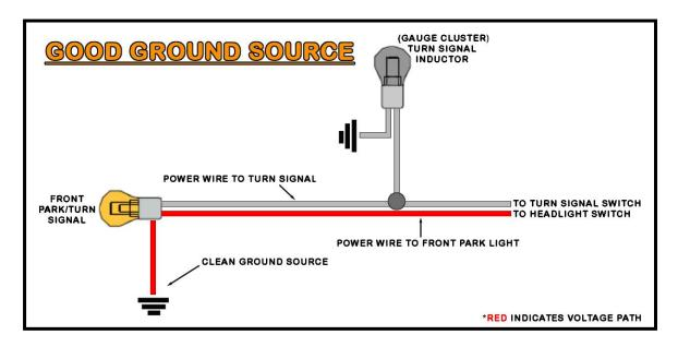
When a ground is not connected properly or is contaminated with dirt, corrosion, or paint, the current will then find the easiest path to ground. This is represented in the diagram below.
