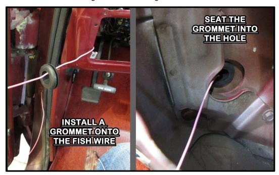
3. Loop the end of the fish wire nearest the grommet with the end of WHITE #961. Make sure that neither the fish wire nor WHITE #961 is wrapped around the dash or emergency brake. Also make sure you tape the ends of the wire as shown. This will prevent wires catching anything as you pull the wire through the door jamb.
