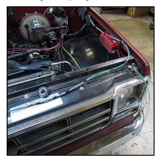
• Route the wires for the passenger side lights across the core support to the right side of the vehicle. The factory ran these wires two different ways:
