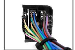
In order to utilize these switched power sources, you must add wires to the engine harness bulkhead. Terminals have been provided in the parts kit for these connections (see page 22). These terminals will accept 18-14-gauge wire, using a 1/4" strip length, and are easiest to install with a non-insulated terminal crimp tool, shown on page 4, and demonstrated below.
