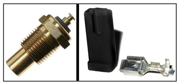
Two-wire temperature sensors on fuel injected engines are for engine computer input, not for gauge signal. Also, if connecting to an engine in a vehicle that has electric cooling fans, make certain you know the difference between the coolant temp sensor and the electric fan thermostatic switch; both of these sensors can look identical.
