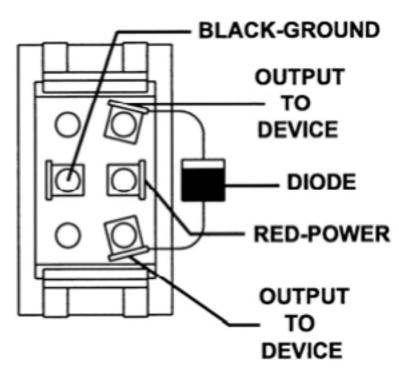
DIODE INSTALLATION: With diode stripe on top (as shown) it will send power out the bottom and top output wires when the top of the switch is pushed, but it will only send power out the top output wire when the bottom side of the switch is pushed. It will be opposite if the diode is reversed.
