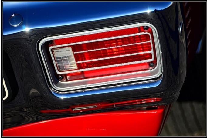
Integrated turn brake signal vehicles will usually have 1 socket per side with a dual filament bulb (brighter filament for turn/brake, dimmer filament for taillights). You can also have vehicles that have integrated lights but also have multiple sockets and lenses.
