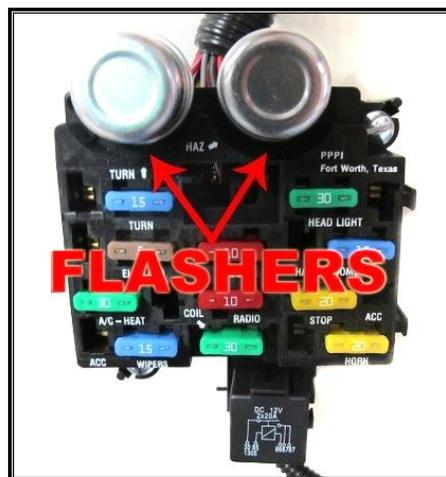
Some LED turn signals do not draw enough current to activate a typical thermal flasher. If you are using LED turn signals, and your turn signals do not work properly and you are certain everything is connected properly, a no-load flasher will be required ([Painless part number #80230](#)).
