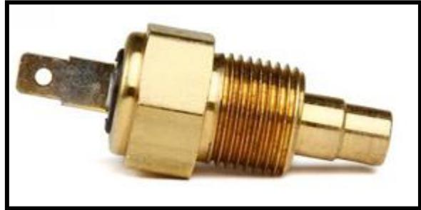
The coolant temp sending unit or temp switch can be mounted in the intake manifold or the side of either cylinder head. These will have a peg, tab, or threaded post to connect to, as seen in the photos on this page. Terminals have been provided for those with the style of sensor seen below. Your factory notched connector will need to be re-used; rolover crimpers will be needed to install this terminal.
