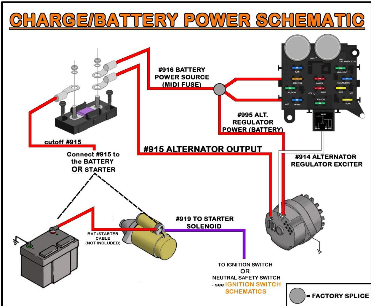
Locate the bag kit provided with the Painless harness kit labeled "ALTERNATOR." This bag kit contains the hardware needed to make the appropriate connections to the alternator as well as a covered inline fuse holder.
