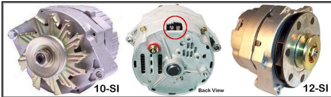
The 10-SI and 12-SI alternators are easy to identify. They have an external fan behind the pulley (the 12-SI has enclosed style fan blades) and a 2-pin connection. This 2-pin connection is circled on the second example in the image above. These are also commonly referred to as “Delco” or “Delcotron” alternators.
