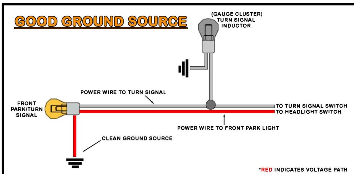
When a ground is not connected properly or is contaminated with dirt, corrosion, or paint, the current will then find the easiest path to ground. This is represented in the diagram below.
