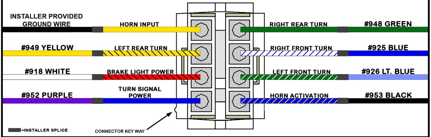
The diagrams above show splicing the wires from the Painless harness to an installer created pigtail from factory wiring.
