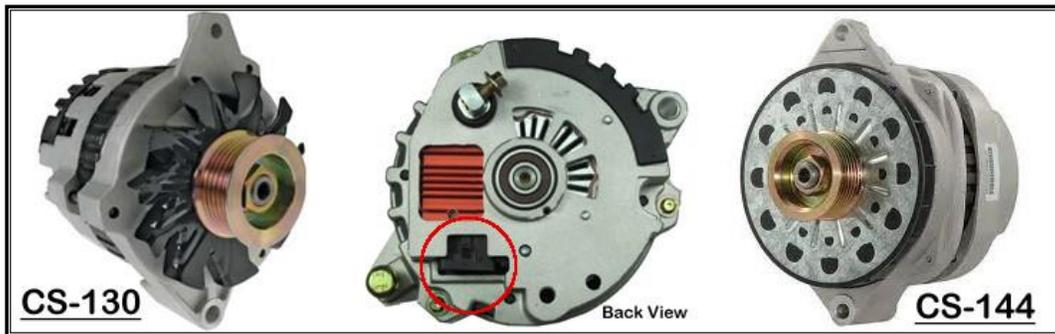
The CS-130, CS-121, and CS-144 alternators closely resemble the SI series alternators. They have an external fan behind the pulley and, generally, a plastic casing on the side and back. These alternators have a 4-pin, sealed connector, shown in the photo below and circled in the image above. The regulator will be marked P, L, S, F. This type of alternator was used on GM TPI and LT1 fuel injected engines among other late 1980s to mid-1990's GM vehicles.
