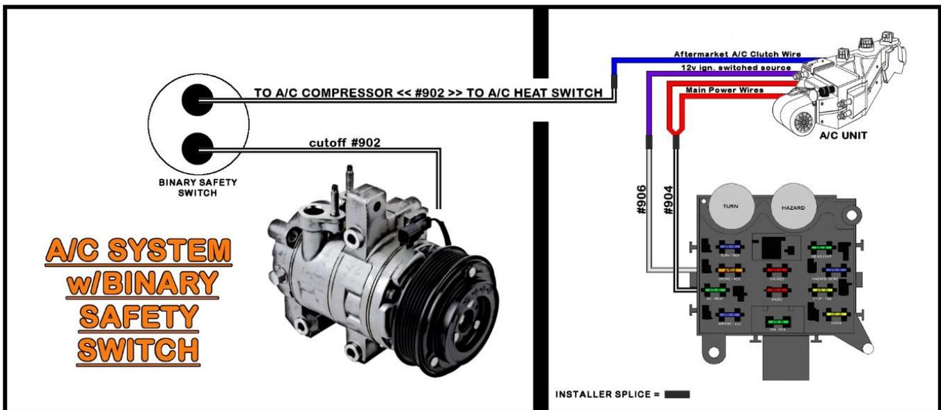
Your aftermarket system should come with all the wiring needed for proper operation. This wiring will need to be connected to power sources provided by the battery and the Painless harness.
