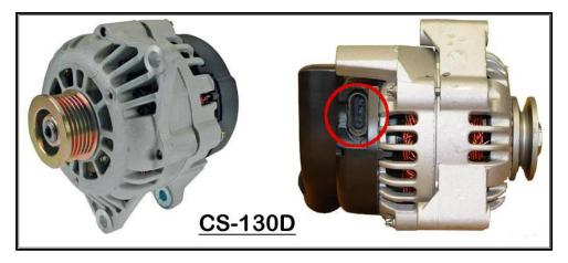
The CS-130D can be spotted by the lack of an external fan behind the pulley. These alternators have an internal fan and a plastic casing on the back. These alternators have an elongated, oval, 4-pin, sealed connector, seen circled in the image above. The regulator will be marked P, L, I, S. This type of alternator was used on many engines, including the GM LS series, Vortec, and Gen. III Vortec truck fuel injected engines.
