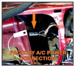
Your factory A/C panel may have a backlight socket. To power this light, it will be necessary for the installer to splice into the BROWN #930 INSTRUMENT PANEL LIGHTING wire in the instrument panel section to provide this power source
