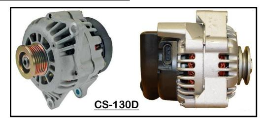
The GM CS-130D can be spotted by its lack of an external fan behind the pulley. These alternators have an internal fan. They also have a plastic casing on the back. These alternators have an elongated oval, 4-pin sealed connector, as seen in the image above. The regulator will be marked P, L, I, S. This type of alternator was used on many engines, including the GM LS series, Vortec, and Gen. III Vortec truck fuel-injected engines.
