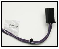
This switch sits in the line of the wire coming from the "Start" terminal of the ignition switch to the "S" terminals of the starter solenoid.
