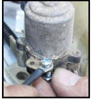
If you are using an aftermarket pump, with two tabs and no separate ground wire hard mounted, and are unsure which tab is power and which is ground, hook it up how you
