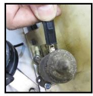
Connect the YELLOW #983 wire to the tab on the wiper pump, the pump can be found on the bottom of the washer fluid reservoir.
