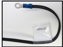
**GROUND**, this wire provides a ground source to the many indicator lights found across the dash through a series of splices. This wire is also doubled up with another #969 wire at this ground connection which makes it part of the integrated ground circuit.
