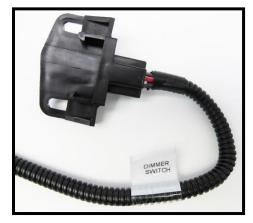
**RED/WHITE**: 14-gauge wire, printed **#907 DIMMER SWITCH POWER**, this comes from the headlight switch and will have power whenever the headlight switch is in the *HEADLIGHT ON* position.
