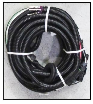
Locate the Engine/headlight harness; this will be the harness with a large rectangular bulkhead connector pre-installed. This harness will have connections for the headlights, horn, front turn signals, and marker lights, as well as connections for components on the engine and for the start, charge, and ignition systems.
