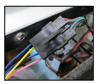
Connect the 4-pin BLACK connector on the wiper switch pigtail to the connector coming from the wiper motor, as seen in the photo.
