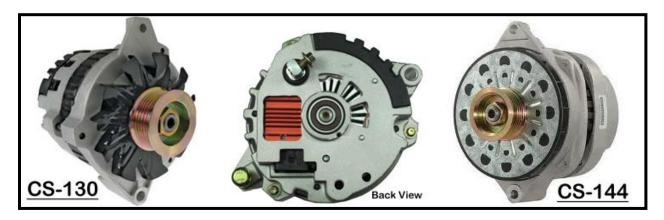
The GM CS-130, CS-121, and CS-144 alternators closely resemble the SI series alternators. They will have an external fan behind the pulley and they generally have some plastic casing on the side and back. These alternators have a 4-pin sealed connector, seen in the photo below and the middle image above. The regulator will be marked P, L, S, F. This type of alternator was used on GM TPI and LT1 fuel-injected engines among other late 1980s to mid-1990s GM vehicles.
