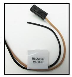
TAN 14-gauge wire, printed #967 BLOWER MOTOR POWER, this wire will supply switched ignition power to the blower motor from the blower motor switch on the dash.
