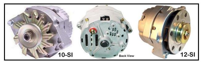
The GM 10-SI and 12-SI alternators are easy to identify. They will have an external fan behind the pulley, the 12-SI having enclosed style fan blades, and a 2-pin connection. This 2-pin connection can be seen in the middle image in the diagram above. These are also known as "Delco" or "Delcotron" alternators.
