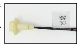
This connection will provide power and ground to the left/driver-side park light. This is a 2-wire molded connector, these wires are:
