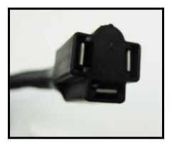
wire will have power when the dimmer switch is in the high beam position and the headlight switch is in the headlight ON position. There is another GRAY/RED #908 doubled up with this wire, this other wire feeds high beam power to the passenger side headlight.
