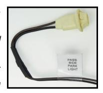
WHITE: 18-gauge wire, printed "#929 PARK LIGHT POWER", this wire will provide power to the park light when the headlight switch is pulled to the "PARK/TAIL LIGHT ON" or the "HEADLIGHTS ON" positions. This WHITE wire comes from a splice which also provides power to the tail lights and the passenger side park light, as shown in the Tail Harness Schematic on page 139. This WHITE wire splices to a BROWN wire coming from the molded light socket, also seen in the Tail Harness Schematic.
