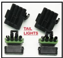
• A molded 4-pin connector pigtail can also be found. This connector is to allow connection to the trailer connector found on the tail harness. This connector will help provide power for left and right turn/brake lights, tail lights, and ground to a trailer. This connector can also allow those who flat tow their Jeep a connection to provide power to the rear lighting of the Jeep. This connector and its use are described in detail beginning on page 134.
