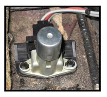
Your headlights will not function unless the dimmer switch connector is connected to a functioning dimmer switch.
