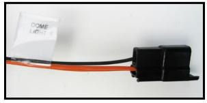
install Painless part #30710 (a universal courtesy light kit) if under-dash lighting is desired.
