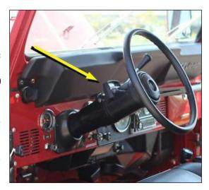
Locate the turn signal connector on the column and plug the connector on the new Painless harness into this connector. It will only connect in one way.
