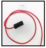
**BLACK**: 16-gauge wire printed with #969 HORN GROUND; this wire will provide the Hom with a ground source. This wire is part of the integrated ground circuit in this harness; it can be seen in the <u>Engine Harness Grounds Schematic</u> on page 12. This wire will be open-ended and may not be needed on most applications.
