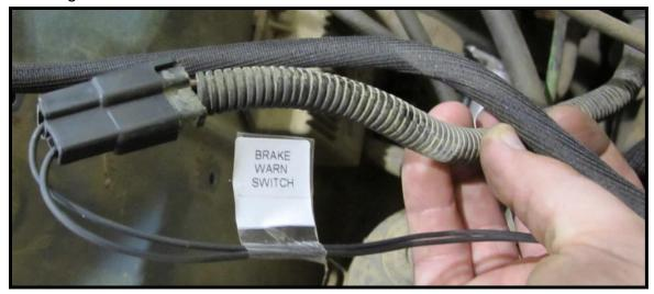
For those with a single-pin brake warn switch; a pigtail to the single-pin switch will be needed.
