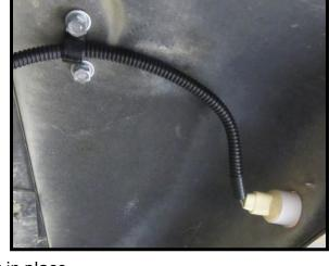
• In the bag kit, you will notice 2 steel & rubber clamps, these clamps are for the driver and passenger side marker light wiring. These clamps will keep the wiring and conduit from sagging. Use the bolts holding the hood catch to mount the clamp.
