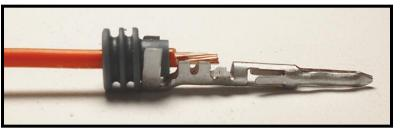
the middle of the terminals should cradle the exposed copper of the stripped wire. If things do not fit as shown, you may have too much exposed copper wire or not enough. You will need to adjust your strip length until your terminal, seal, and wire strip resemble those pictured. Failure to do so will result in a bad crimp.
