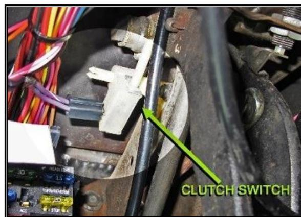
Re-use the connector from the factory harness, seen to the right, or use the small insulated terminals that have been provided in the parts kit. It does not matter which tab each wire connects to. Once connected to the switch, route the cutoff portion of **#919** to the ignition switch. The ignition switch connection will be covered in the next section.
