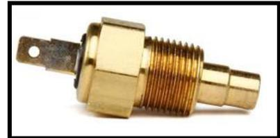
The coolant temp sending unit or temp switch can be mounted in the intake manifold or in the side of either cylinder head. These will have a peg, tab, or threaded post to connect to, as seen in the photos on this page. Terminals have been provided for those with the style of sensor seen below. Your factory notched connector will need to be re-used; rollover crimpers will be needed to properly install this terminal.
