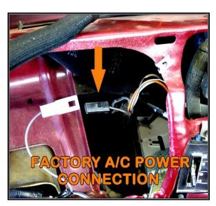
Locate the inline connector on the factory heat or A/C harness, it will be a single-pin connector with a BROWN wire several inches away from the blower switch connection. Plug the BROWN #904 power wire into this connector on the air conditioning harness.
