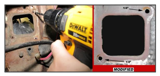
With the bolt holes drilled to 1/4" in the firewall, the fuse block can now be mounted.
