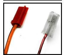
Using the terminal removal procedure, found on page 22, remove the two fuse block connectors on the factory harness. Remember to pry the locking tang of the terminal back out once the connector is removed. The factory connectors can also be cut from the original harness and the new terminals that are provided with the Painless kit can be installed.
