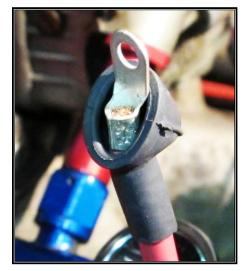
ONE WIRE ALTERNATOR, meaning it does not require a switched 12v source or regulator connections, or if the Painless or other aftermarket fuel injection harness you are using has an alternator connector, then this output wire is the only wire used in this section at the alternator.
