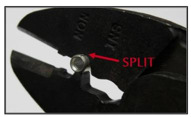
"Umbrella" style zip-tie clips have been provided for you to attach the Painless harness to the inner fender, core support, and/or frame. These zip-tie clips fit into 1/4" holes left behind by factory plastic retainer loops or those created with a drill by the
