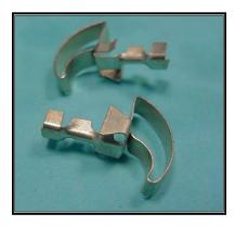
Those with spring/contact sockets must reuse the factory springs and socket. Before cutting the factory socket from the harness, take note as to what color wire went into each location, so you know how to install the new wires. When installing the socket to the Painless harness, first, install the wires into the socket. Next, install the spring, and in some cases, a plastic disk, then install the terminal and pull the assembly down into the socket.
