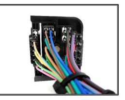
If any wires were added to the bulkhead connector, group each wire with the section of **Engine Harness** nearest to where the fuse will be installed. For instance, if you are mounting an inline fuse on the driver side inner fender to power an accessory, the wire leading to it will route with the **Front Light Section**.
