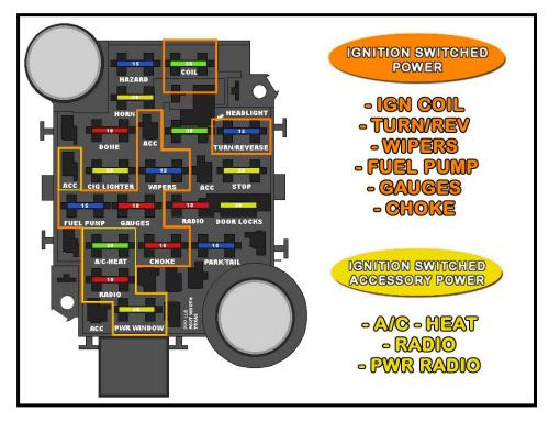
The drawing above shows all the switched ignition fuses. These fuses are powered by wires coming from the ignition switch (wires **#931**, **#932**, and **#933**) and receive power depending on what position the ignition switch is in. None of these fuses should have power when the ignition is in the *OFF* position. The <u>Ignition Switch Section</u> beginning on page 90 of this manual will go into further detail about power supplied to these fuses.
