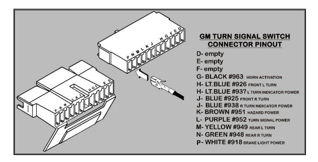
• Those with a factory 1968 or earlier columns, terminals, as shown below, are provided for you to reuse the factory "semi-circle" turn signal connector from the old harness. This is done by using a small flat screwdriver or stiff piece of wire and flattening the locking tangs on both sides of the terminal to remove them from the connector, as shown in the photos below.
