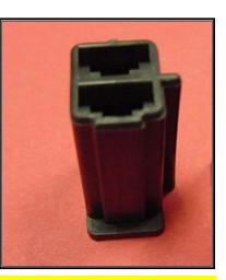
If you do not have a neutral safety/clutch switch and do not plan on getting one, connect these 2 PURPLE #919 wires together.
