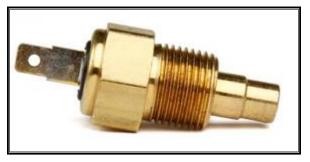
The coolant temp sending unit/switch can be mounted in the intake manifold or the side of either cylinder head. These will have a peg, tab, or threaded post to connect to, as seen in the photos on this page. Terminals and a factory-style connector have been supplied to allow connecting to a factory-style sensor, rollover crimpers will be needed to install this terminal.
