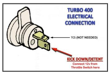
• If you have a factory, pedal mounted accelerator switch, you can use a switched power source inside the vehicle or you can route the cut off piece of **#954** to the interior, connect at the throttle switch, and then route it back out to the transmission.
