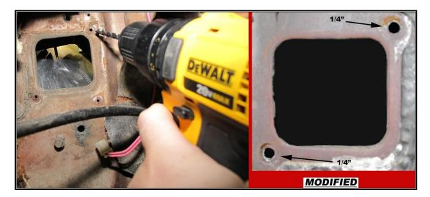
With the bolt holes drilled to 1/4" in the firewall, the fuse block can now be mounted.
