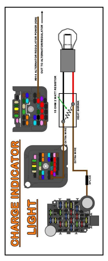
The remaining alternator connections vary based on which alternator is being used. Choose the alternator that best represents the alternator found on your vehicle from those on the next few pages. Then, follow the instructions provided for your alternator.
