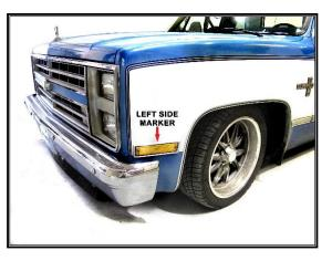
The park light feature is activated by a power source coming from the headlight switch. This light illuminates any time the headlight switch is in the "PARK" or "ON" position. The turn signal feature is provided by a power source coming from the turn signal switch.
