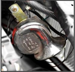
• If you have a tab on the horn, locate the terminal and connector, seen below, provided in the parts kit.
