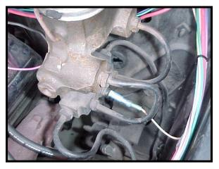
**Note:** This is a pressure switch, not a fluid level switch. This switch is only necessary if you want the brake warning light in the dash to indicate low brake fluid pressure. If you have aftermarket gauges without a brake warning light, this connection can be skipped, and this wire can either be removed from the harness.
