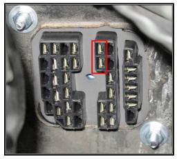
The ignition switched power on these (2) pins comes directly from the ignition switch. These pins
