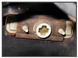
• Using splices and heat shrink from the parts kit, connect the **#926** and **#927** wires to the lamp socket. Double up with the cut off pieces to allow connection to the front turn/park light as shown in the diagram below.
