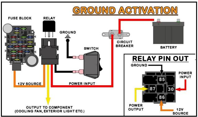
A <u>ground activated relay</u> is just the opposite of the 12-volt activated relay; 12 volts (battery constant or switched) are supplied uninterrupted and the ground wire is switched. The Horn Relay pre-wired in the Painless harness is a Ground Activated Relay. Another example of this method is a thermostat operated fan relay. In this case, however, a thermostatic switch would replace the switch in the drawing above (see below).
