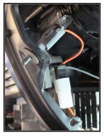
• With the factory switch now modified, install it into the dash and connect it to the **ORANGE #971** wire on the Painless harness.
