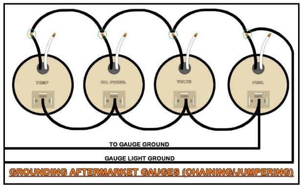
Gauge light power is supported by the **GREY #930** wire. This wire connects to one of the leads for the gauge light or the gauge light tab found on gauges with LED backlighting. To make these connections you can splice from this **GREY #930** wire to all the gauges or chain/jumper it all together.
