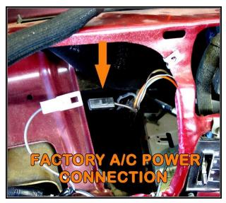
Locate the inline connector on the factory heat or A/C harness, it will be a single-pin connector with a BROWN wire several inches away from the blower switch connection. Plug the BROWN #904 power wire into this connector on the air conditioning harness.
