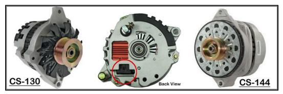
The CS-130, CS-121, and CS-144 alternators closely resemble the SI series alternators. They have an external fan behind the pulley and, generally, a plastic casing on the side and back. These alternators have a 4-pin, sealed connector, shown in the photo below and circled in the image above. The regulator will be marked P, L, S, F. This type of alternator was used on GM TPI and LT1 fuel injected engines among other late 1980s to mid-1990s GM vehicles.
