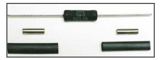
\*In factory applications where this alternator was used, a charge indicator light created the necessary resistance. For those with an instrument panel with a charge indicator light, the resistor is not needed. However, the **#914** wire needs to be routed to one side of the charge indicator light and the other side of the light then routes out to the alternator. A charge indicator light was explained in more detail on page 53.
