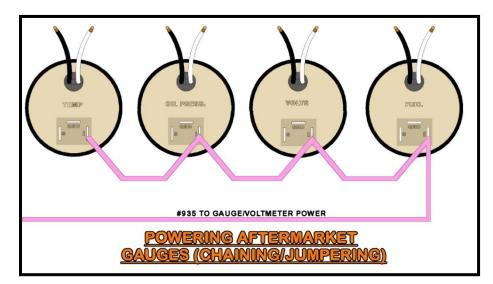
Grounds need to be supplied to the gauge lights and any ground tab on the gauges. The installer needs to run a ground circuit for gauge connections. To make these ground connections you can splice from the installer provided ground wires to all the gauges or chain/jumper it all together. Both methods can be seen in the following two drawings:
