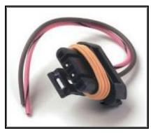
Without this resistance, the regulator on the alternator will burn up. The resistor simply needs to be installed inline on the pin "L" wire, **#914**, as shown in the diagrams on the next page.
