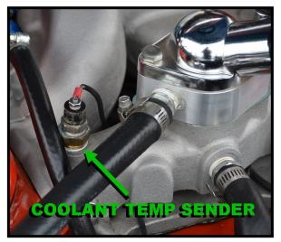
• Route this **GREEN #921** wire to the coolant temp sensor, cut to length, strip <sup>1</sup>/<sub>4</sub>" insulation, and crimp on the appropriate terminal for your connection, and connect.
