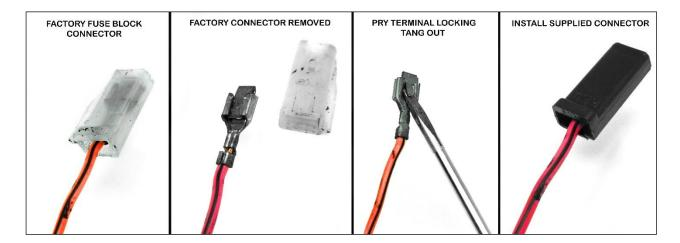
Install one of the single-pin connectors on each of the factory wires and connect them to the Painless harness. The factory pink/black wires connect to the power window, YELLOW #913 wire on the Painless harness. The factory, orange/black wire connects to the power lock, YELLOW/BLACK #912 wire on the Painless harness.
