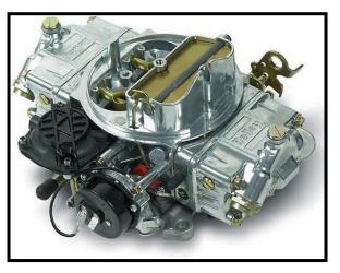
as it is heated causing the choke to slowly open. When the ignition is turned to the "OFF" position, power is no longer on this wire, causing the spring to begin to cool and contract, closing the choke.
