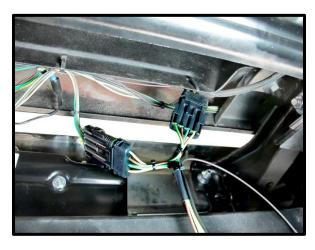
**Step 4:** Finally, attach the ground wire to reliable ground using the hardware provided.
