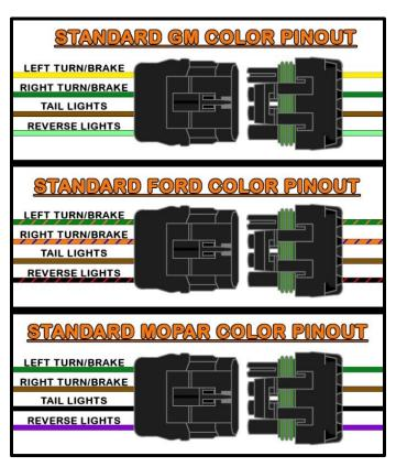
Step 1: Locate the 4 wires in your harness you will need: The Left Turn/Brake, Right Turn/Brake, Tail Lights, and Reverse lights wires. Though these colors vary by make the standard colors can be seen in the diagram to the left.
