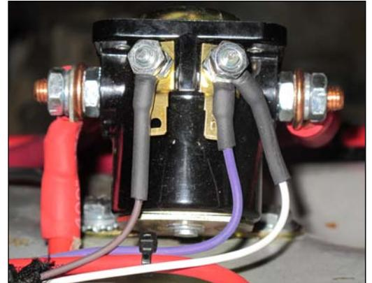
7. Connect the brown wire, printed "**POWER IN START/CRANK-"I" TERMINAL ON SOLENOID**" to the "I" terminal of the starter solenoid. This wire will provide what is known as a "Ballast Bypass" to provide the coil a full 12v source at start up.
