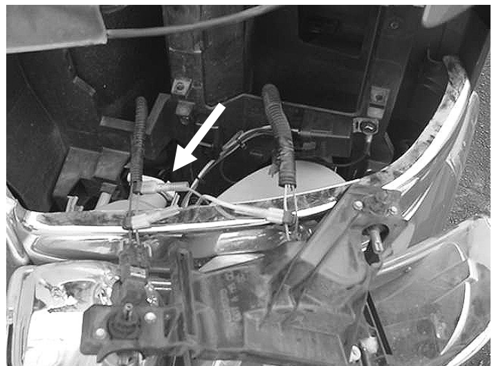
Illustration #4 The orange wire from relay has been terminated and T-tapped to the orange headlight wire.
