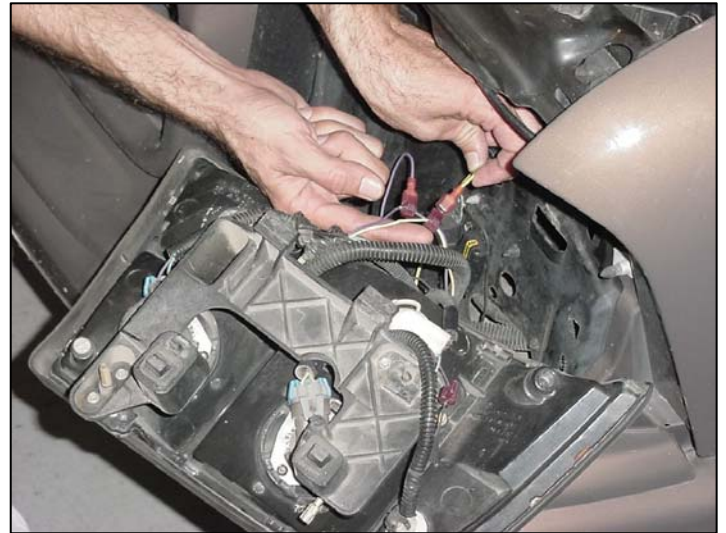
Illustration #3 Installing the T-Taps
