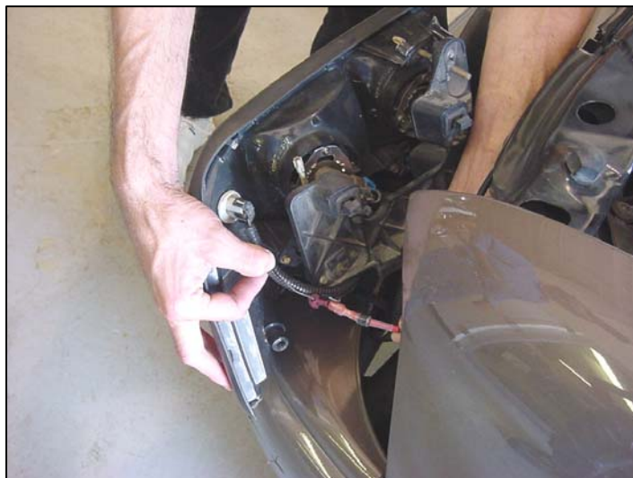
Illustration #4 Connecting the Power Source
