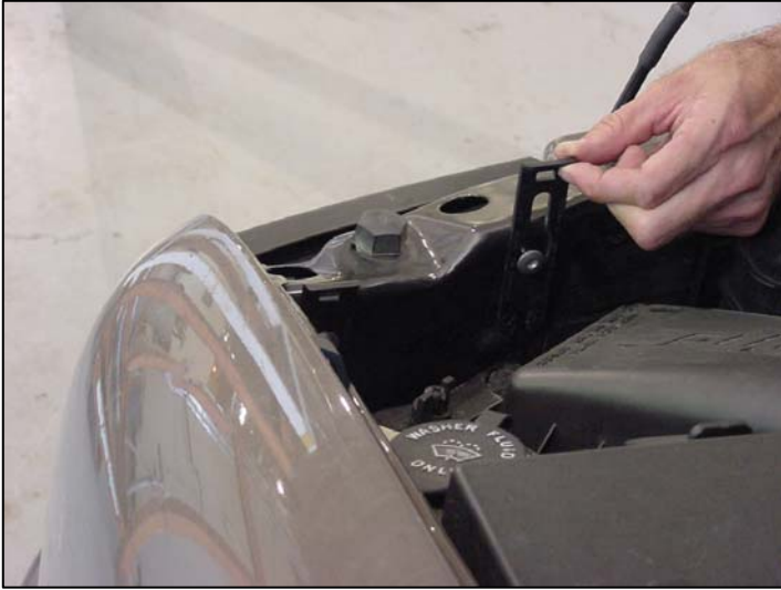
Illustration #1 Head Light Retainer Clip & Head Light Removal
