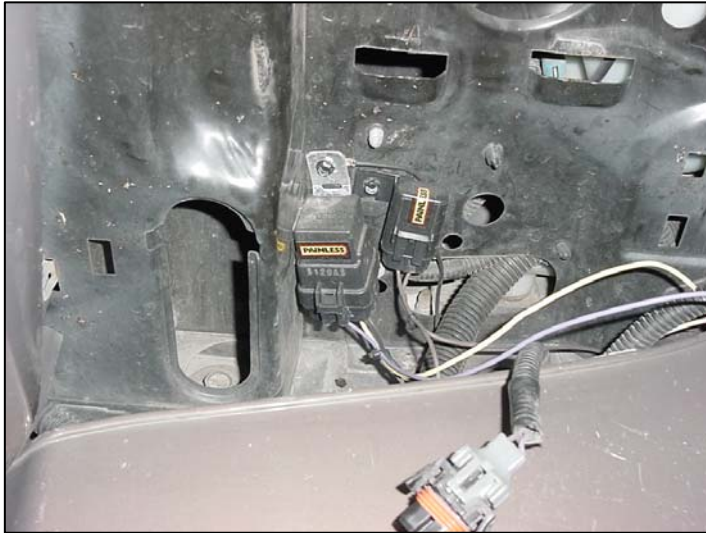
Illustration #2 Mounting the Relay & Fuse
