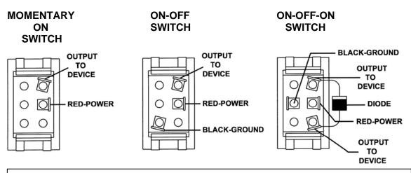
DIODE INSTALLATION: With diode stripe on top (as shown) it will send power out the bottom and top output wires when the top of the switch is pushed, but it will only send power out the top output wire when the bottom side of the switch is pushed. It will be opposite if the diode is reversed.
