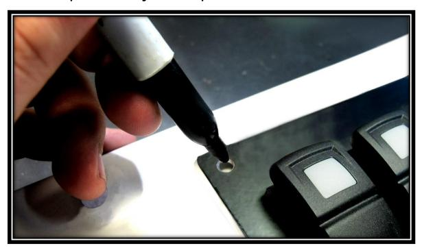
Step 8: Remove the Switch Panel and use a <sup>13</sup>/<sub>64</sub>" or #7 drill bit to create the (4) mounting holes.
