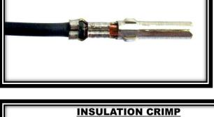
• With Strap 1 crimped, move onto crimping the insulation strap: Strap 2. Place Strap 2 into the appropriate iaw of
