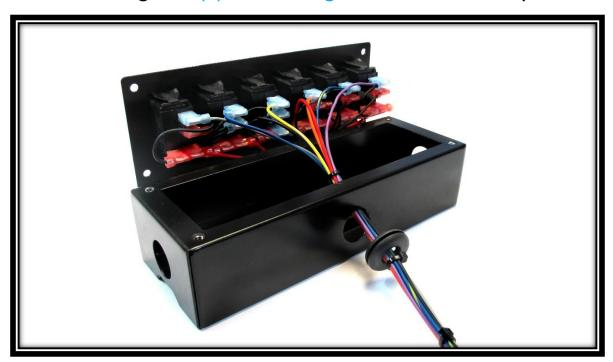
Step 7: At this point you may choose to loom the Switch Panel Wires. We recommend Painless ½" PowerBraid (P/N: 70902). Run the loom over the wire, through the grommet, and into the box. You can secure the end of the loom with a zip-tie. Note: It isn't necessary to loom the entire wiring harness as you will cut these wires to length later. Simply loom a few feet and make sure the end inside the base is secure.
