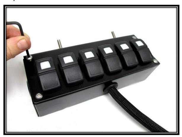
Step 10: Line up the bolts you inserted into the Switch Panel's mounting bracket in Step 4 with the holes you drilled out in Step 2. Attach the Switch Panel using (2) 1/4" lock nuts found in the
