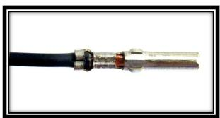
• Using the appropriate jaw on the crimpers, crimp Strap 1. The appropriate jaw depends on the wire gauge as well as the terminal stiffness. If you are unsure which jaw to use, you can always start with the biggest and work your way down until you get a tight crimp.
