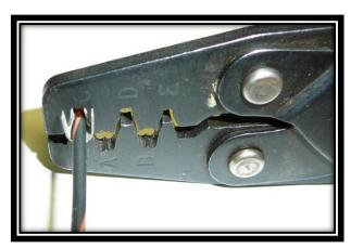
• Insert the wire into the terminal. There are two terminal straps on the terminal. For instructional purposes, we will label them 1 and 2. Strap 1 crimps the exposed copper strands of the wire, while strap 2 crimps the wire insulation. Make your strip length long enough to ensure only copper strands are crimped by Strap 1 but short enough that only insulation is crimped by Strap 2. The photo to the left best demonstrates this.
