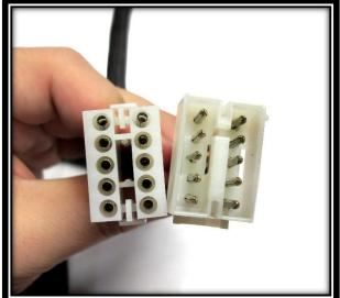
**Step 18:** Link the two connectors and join the wiring harness from the **Fuse/Relay Center** to the **Switch Panel**. Use **zip-ties** to secure the wires up under the dash and out of the way.
