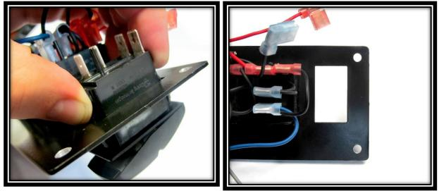
**Step 21:** Insert the **Momentary On Switch** into the empty socket of the bracket. Then, connect the ground and output wires. The red wire will not be needed and can be stowed out of the way.
