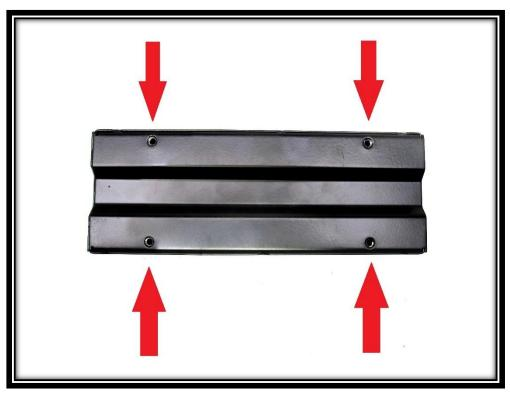
Step 9: Then, select (4) #10 lock washers, (4) #10 flat washers, and (4)  $10 - 32 \times \frac{3}{8}$ " button head screws and the small hex key provided in order to mount the Switch Panel.
