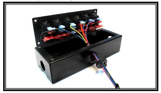
Step 4: If you wish to loom the Switch Panel Wires, do so now. We recommend Painless ½" PowerBraid (P/N: 70902). Run the loom over the wire, through the grommet, and into the box. You can secure the end of the loom with a zip-tie. Note: It isn't necessary to loom the entire wiring harness as you will cut these wires to length later. Simply loom a few feet and make sure the end inside the base is secure.
