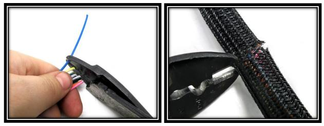
Step 14: Strip each of the Switch Panel Wires <sup>3</sup>/<sub>16</sub>", and install a female pin terminal from the parts kit onto the end of each wire. See page 3 for detailed instructions on how to properly crimp these terminals. We recommend Painless #70900 Roll-Over Crimpers.
