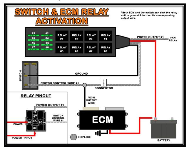
**Step 25**: Then, splice the ECM Output wire into the **Switch Control** wire of the switch you wish to use. See page 9 for the wire color chart.
