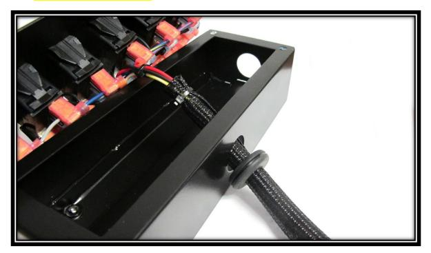
Step 5: Place the rubber grommet into the opening. Then, use the (2) plastic plugs provided in the parts kit, to close up the remaining holes.
