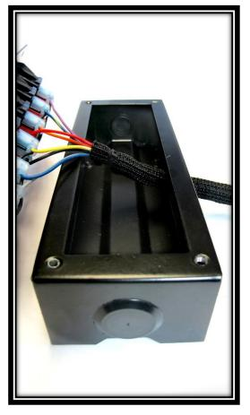
Step 6: Make sure the Switch Panel Box is properly covering the back of the Switch Panel, and use (4)  $10 - 32 \times \frac{3}{6}$ " button head screws and the small hex key provided in the parts kit to secure the panel to the box. Remember to start each screw into the threads and tighten evenly.
