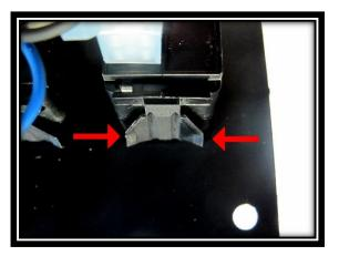
**Step 20:** These tabs lock the switch in place. To remove the switch, squeeze the tabs in and slide it out of the bracket.
