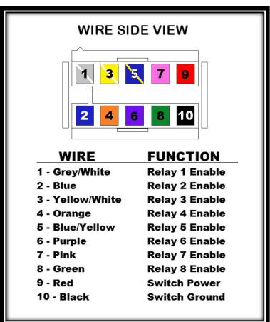
Step 13: After routing the Switch Panel Wires to the Fuse/Relay Center's Switch Control Wires, cut the Switch Panel Wires and loom (if used) to length. Secure the end of the loom with a zip-tie (provided) or a large piece of heat-shrink (not provided).
