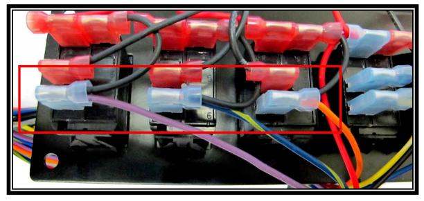
**Step 23:** Therefore, we recommend splicing an additional switch control wire into the switch before the terminal.
