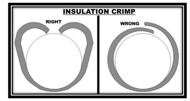
In the parts kit, you will see uninsulated female terminals. These terminals are for the **10-pin connector shell** included in the **Track Rocker Fuse/Relay Center** parts kit, and require roll over crimpers.
