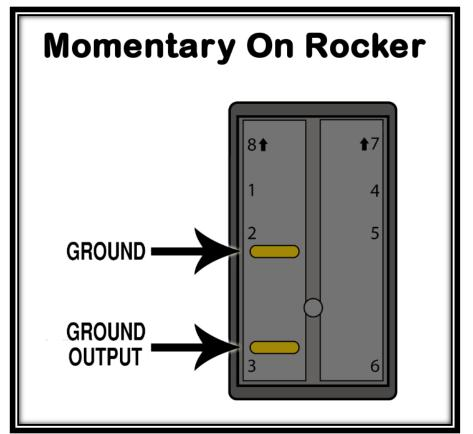
Step 19: To replace a switch with the Momentary On Switch, remove the power, output, and ground wires from the switch you are replacing. Then, locate the tabs located at the top and bottom of the switch.
