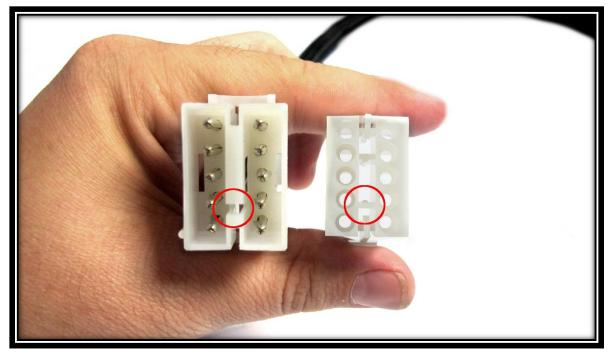
Step 16: Insert the newly pinned wires into the 10-pin connector housing. Make sure, while inserting the pins, that once connected the wire color matches the one across from it. The diagram on page 9 illustrates the pinout of the 10-pin connector housing from the wire side.
