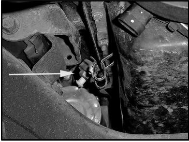
FIGURE 6.5 Knock Sensor Connector
