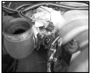
FIGURE 6.12 TPS Sensor and IAC Valve
