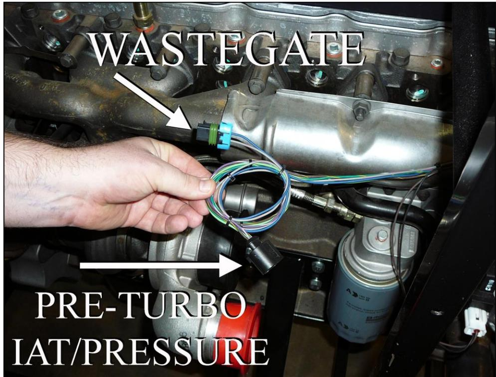
Plug the connector labeled **(PRETURBO IAT/P)** into the pre-turbo intake air temperature and pressure sensor.
