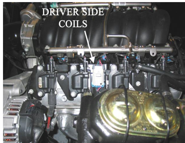
FIGURE 6.18 Driver Side Coil Connector
