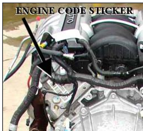
Figure 7.2 Engine Code Sticker
