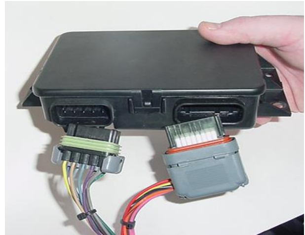
FIGURE 6.22 TAC Module Connections
