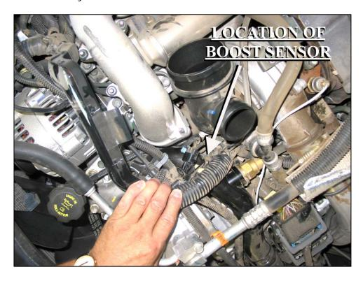
Unplug the factory male boost sensor connector from the boost sensor. Connect the factory male boost pressure sensor connector to the female boost pressure sensor connector on the Striker harness. Connect the Striker harness male boost pressure sensor connector to the boost pressure sensor. Reinstall the wire harness bracket and nut onto the intake tube.
