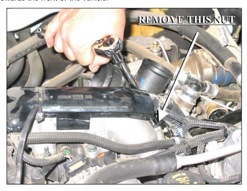
The boost sensor is buried down in the engine valley. The engine must be cool in order to reach the boost sensor connector with your hand.
