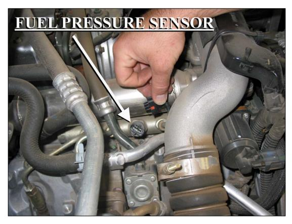
Connect the factory fuel pressure sensor connector to the corresponding female connector on the Striker harness. Connect the male fuel pressure sensor connector on the Striker harness to the fuel pressure sensor.
