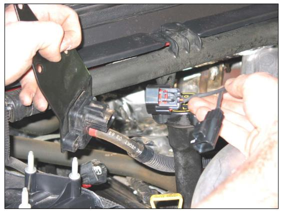
Connect the ground eyelet to this grounding point in the engine compartment. If your harness does not have a ground wire, skip this step.
