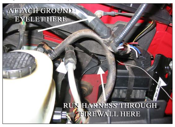
Drill a hole in this plastic cover big enough to accommodate the connector on the harness. Insert the harness through this plastic cover and into the driver's compartment.
