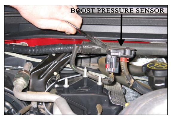
Connect the factory male boost pressure sensor connector to the female boost pressure sensor connector on the Striker harness. Connect the Striker harness male boost pressure sensor connector to the boost pressure sensor.
