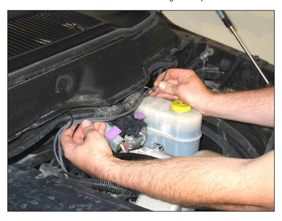
Attach the ground eyelet to this grounding point. If your harness does not have a ground wire, skip to the next step.
