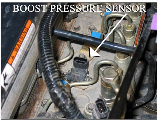
Connect the factory male boost pressure sensor connector to the female boost pressure sensor connector on the Striker harness. Connect the Striker harness male boost pressure sensor connector to the boost pressure sensor.
