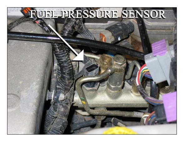
Disconnect the factory fuel pressure sensor connector from the fuel pressure sensor. Plug this male connector into the Striker harness female fuel pressure sensor connector. Plug the Striker harness male fuel pressure sensor connector into the fuel pressure sensor.
