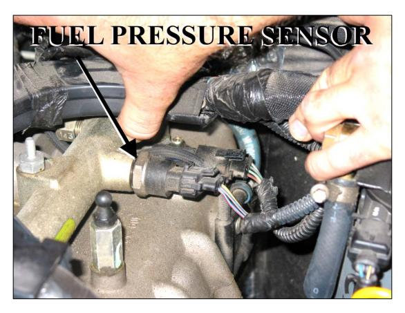
Disconnect the factory fuel pressure sensor connector from the fuel pressure sensor. Connect the factory fuel pressure sensor connector to the corresponding female connector on the Striker harness. Connect the male fuel pressure sensor connector on the Striker harness to the fuel pressure sensor.
