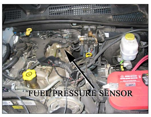
Locate the fuel pressure sensor connector.
