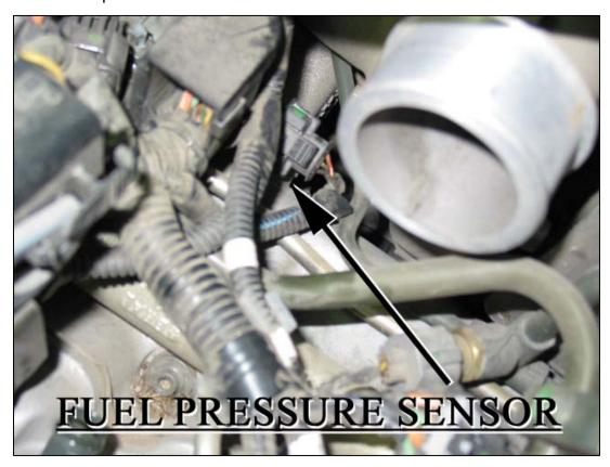
Connect the factory fuel pressure sensor connector to the corresponding female connector on the Striker harness. Connect the male fuel pressure sensor connector on the Striker harness to the fuel pressure sensor. Reconnect the intercooler boost tube and tighten the clamp.
