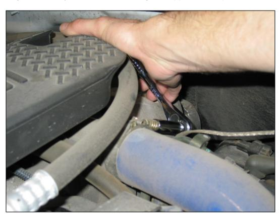
Locate the fuel pressure sensor connector. Disconnect the factory fuel pressure sensor connector from the fuel pressure sensor.
