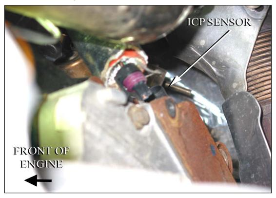
Most late 2004 and newer trucks have the ICP sensor mounted on the passenger side valve cover. Route the ICP sensor connectors on the Striker harness over to the passenger side valve cover. Unplug the male factory ICP sensor connector and connect this to the female ICP sensor connector on the Striker harness. Plug the Striker harness male ICP sensor connector into the ICP sensor on the valve cover.
