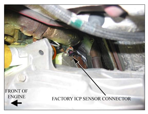
Disconnect the factory ICP sensor connector. Plug this male connector into the female ICP connector on the Striker harness. Plug the male ICP connector on the Striker harness into the ICP sensor. Reinstall the turbo charger heat shield.
