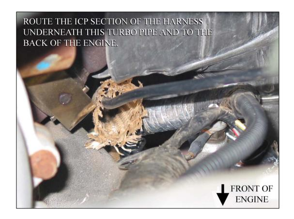
2003 and some early 2004 trucks require reaching up behind the engine and transmission from underneath the truck, on the driver's side, to reach the ICP Sensor connector. Remove the turbo charger heat shield.
