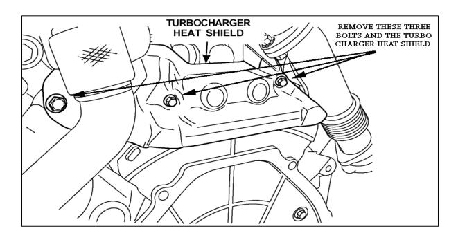
Behind the turbo charger heat shield the ICP sensor can be found mounted into the engine. The factory ICP sensor connector will have insulation surrounding it and the wires from it. This insulation must be pulled back in order to reach and unplug the factory ICP sensor connector.
