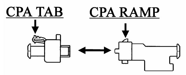
NOTE: Illustration shows correct orientation of connector latch
