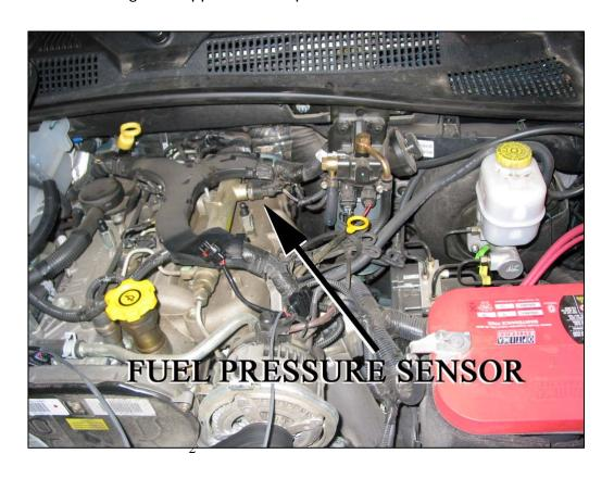
Locate the fuel pressure sensor connector.
