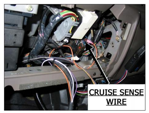
Route and secure the harness up to where the TC controller will be mounted. Plug in the TC module to the harness.
