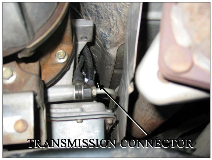
On top of the transmission and towards the back of it is the output shaft speed sensor. Use one of supplied the Posi-Tap connector to attach the green wire, labeled OSS, in the Striker harness to the Dark Blue/Yellow wire in the output shaft speed sensor. See diagrams below. Posi-Tap instructions on page 7.
