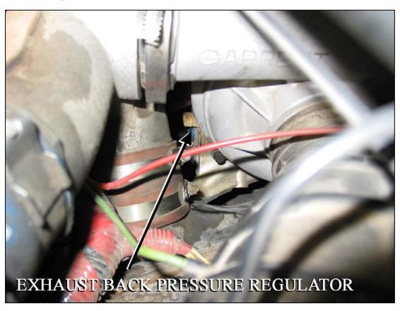
Plug the male connector on the factory harness into the female exhaust brake connector on the Striker harness. Use a tie wrap to ensure these plugs stay together.
