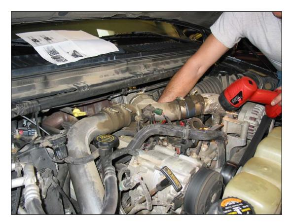
Plug the Striker harness male exhaust brake connector into the exhaust backpressure regulator. Turbo chargers get extremely hot; make sure to route wires away from touching any turbo charger piping or exhaust piping.
