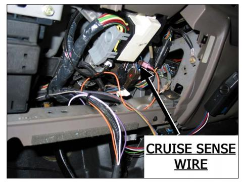
Route and secure the harness up to where the EB controller will be mounted. Plug in the EB module to the harness.
