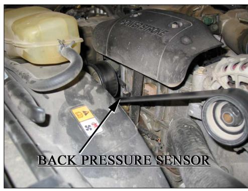
Next, unplug the factory connector from the sensor. Plug in the eliminator into this factory connector. Use a tie wrap to hold the connector and eliminator away from the belt and pulleys.
