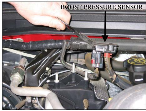
Next, unplug the factory connector from the boost sensor. Plug in the male connector side of the Overboost code eliminator into this factory connector. Finally plug the factory connector into the female connector side of the Overboost code eliminator.
