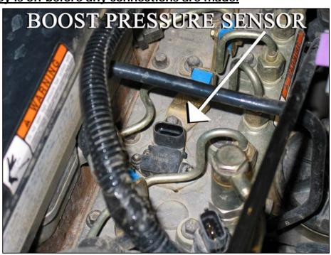
Next, unplug the factory connector from the boost sensor. Plug in the male connector side of the Overboost code eliminator into this factory connector. Finally plug the factory connector into the female connector side of the Overboost code eliminator.
