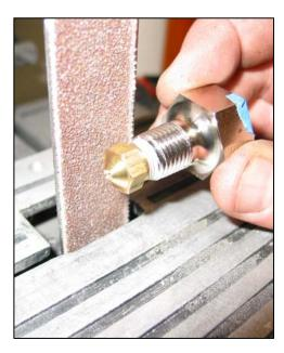
NOTE: Loctite (blue type) the nozzle into the nozzle adapter once you have finalized tuning.
