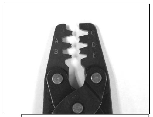
Roll-crimp style terminal crimpers available at your local RadioShack or www.delcity.net part# 990170
