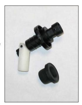
Drill a 13/16" hole where you want the level sensor mounted. Insert the grommet into the hole and then insert the level sensor into the grommet. The white float should droop down towards the bottom of the tank when the tank is empty. You may have to use some light oil to lubricate the level sensor when you insert it into the grommet.
