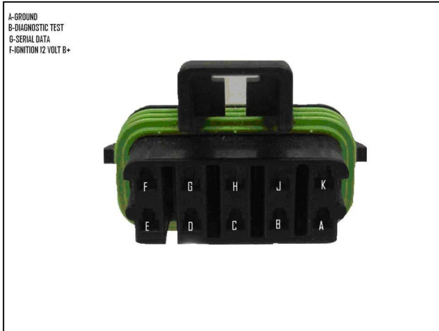
Figure 7.2 Diagnostic Link Connector (DLC)
