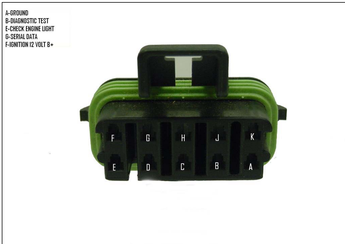
Figure 6.1 Assembly Line Diagnostic Link Connector (ALDL)
