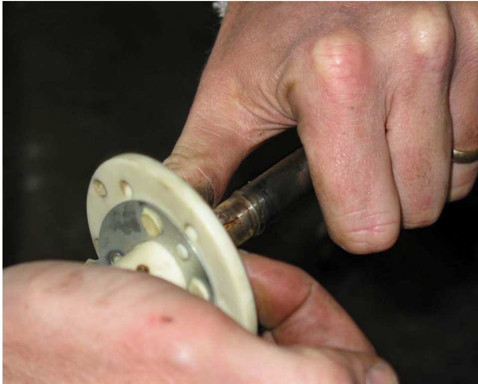
Step #6 Remove the original shutter wheel from the shaft.
